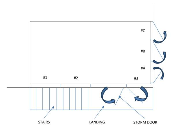
Diagram of the plan view of the porch showing window placement & openings
